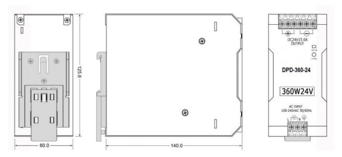
Note: Installation clearances: 40mm on top, 20mm on the bottom, 5mm on the left and right side are recommended when loaded permanently with full power, In case the adjacent device is heat source, 15mm clearance is recommended.
