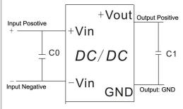
2. Input reflecting ripple current test circuit:
