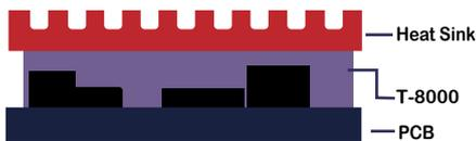
T-8000 offers outstanding thermal conductivity at 15.0 W/m\*K and extremely low thermal resistance under minimal force. T-8000 offers excellent compression, filling small air gaps on uneven surfaces, ensuring an efficient and consistent transfer of heat.
