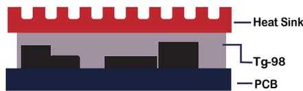
Ts-98 offers outstanding thermal conductivity at 18.0 W/m\*K and extremely low thermal resistance under minimal force. Ts-98 offers excellent compression, filling small air gaps on uneven surfaces, ensuring an efficient and consistent transfer of heat.
